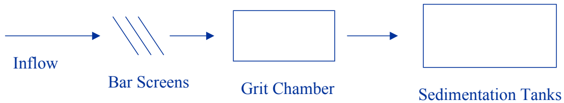
Figure 2-1: Schematic of Conventional Primary Treatment
