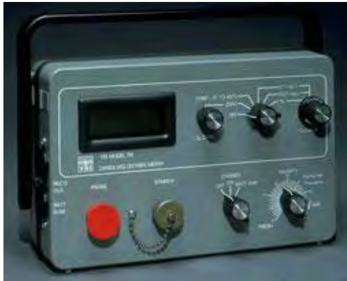
Figure D-3: Portable DO and Temperature meter
