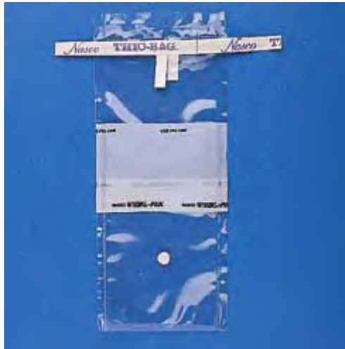
Figure D-2: Whirl-Pak Bag with Sodium Thiosulfate Preservative
