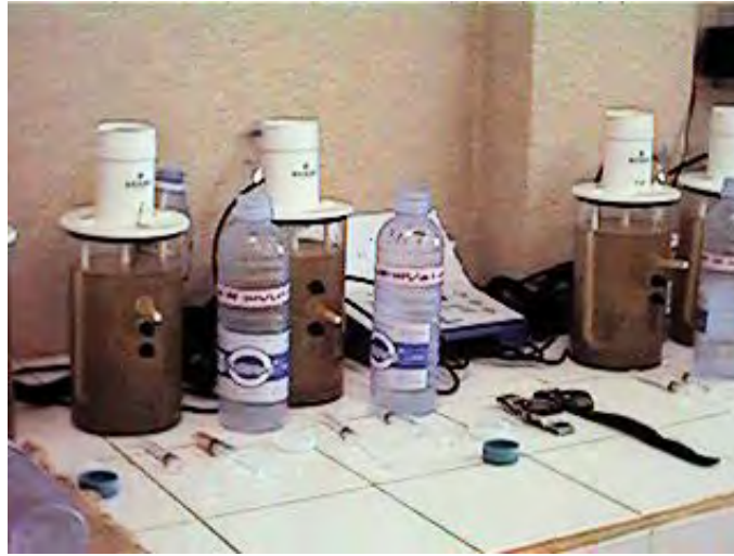
Figure B-4: Jar-testing equipment used on the field study
