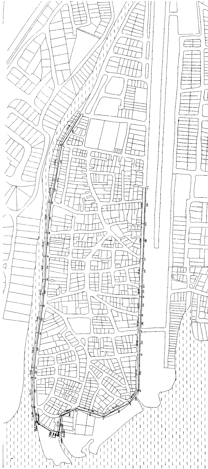
Figure C.1 Trunk Sewer Layout
