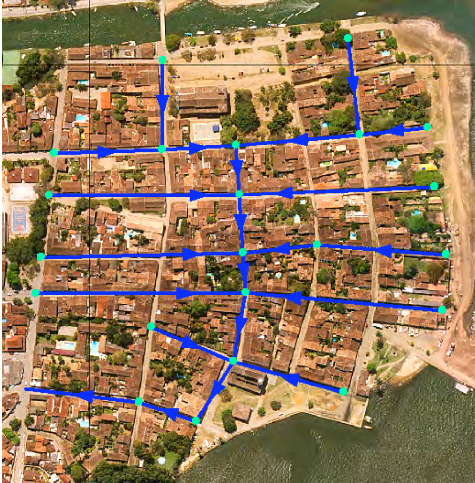
Figure 2: Sewer Network Design
