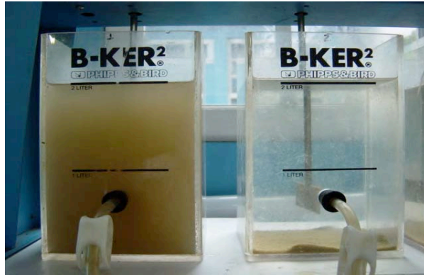
Figure 6.3. Difference in effluent quality
