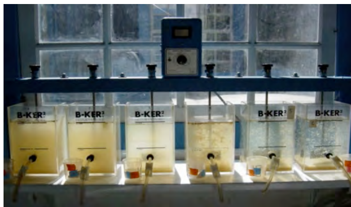
Figure 2.5: Difference in effluent quality due to chemical addition
