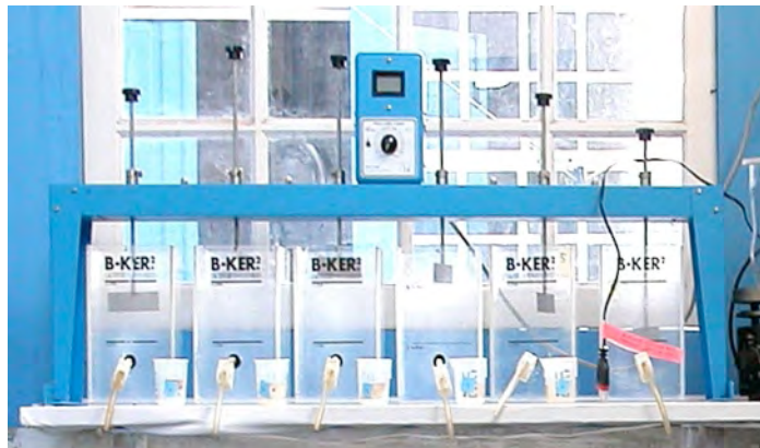
Figure 2.4: Typical jar tests apparatus
