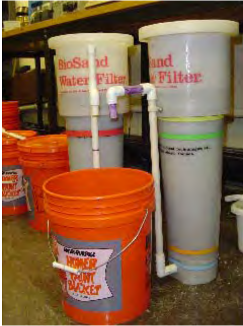
Figure 9.2: BioSand filters setup during laboratory experimentation.
