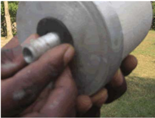
Figure 3.13. Rubber part prevents unfiltered water from leaking in the bottom bucket.
