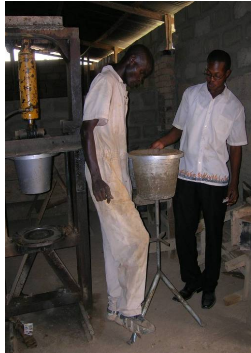
Figure 3.7. Displaying the filter steel mold.
