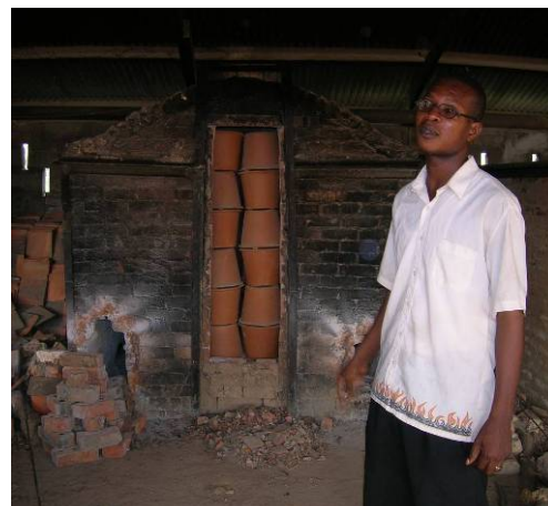
Figure 3.8. Pots stacked inside the kiln before firing.
