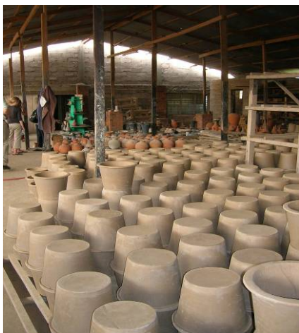
Figure 3.9. Pot filters are dried for several days before firing in the kiln.
