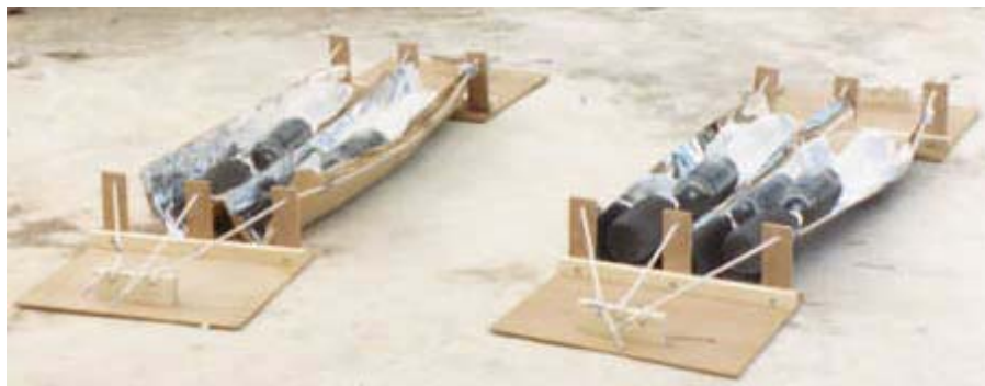
Figure 3.2 Solar reflectors, Left: aluminum foil, Right: aluminum mylar
