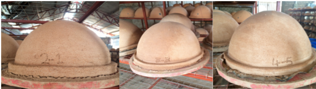
Figure 3-27 Full-sized filters with Three Different Rice Husk Sizes (from left to right: 2-1, 3-3 and 4-5)
