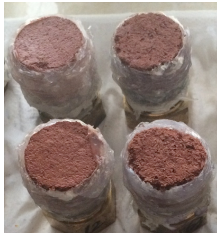
Figure 3-4 Group T F with silicon glue on side faces
