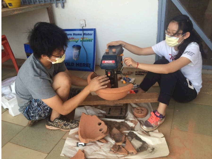
Figure 3-5 The drilling process using a drill press
