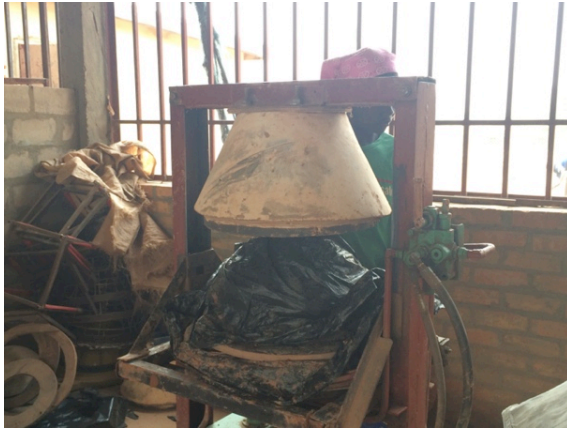
Figure 3-18 The Hydraulic Press showing Male & Female Molds
