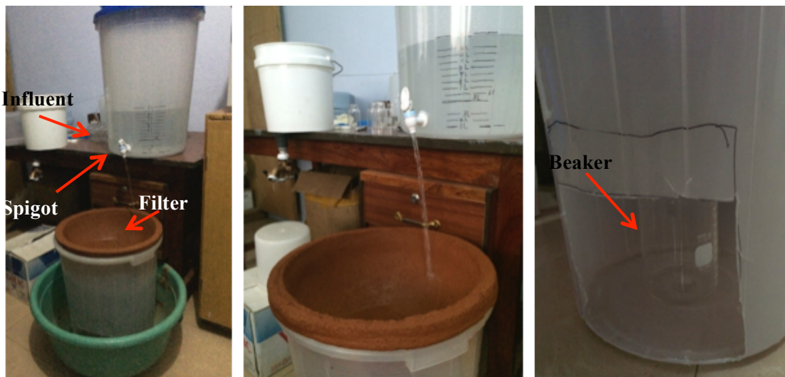
Figure 3-28 The Full-sized Filter Setup at the PHW Lab in Tamale, Ghana
