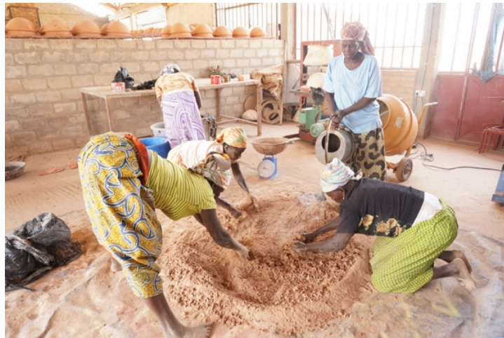
Figure 3-17 Adding water to the mix
