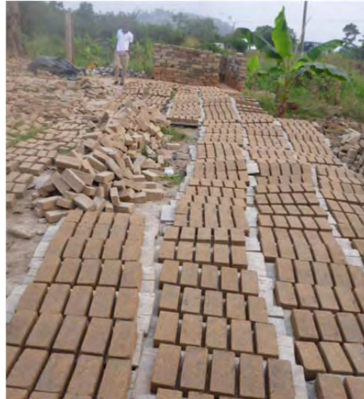
FIGURE 12 - GREEN BRICKS DRYING IN THE OPEN AIR
