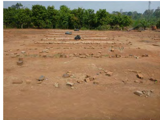
FIGURE 16 - DRYING GREEN BRICKS IN OPEN AIR
