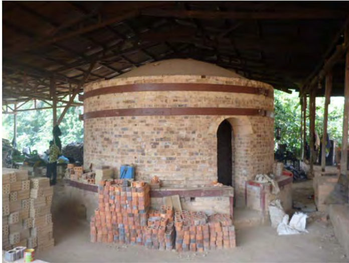
FIGURE 4 - LARGE DOWNDRAUGHT KILN
