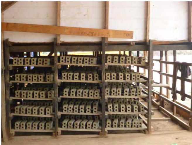
FIGURE 15 - DRYING GREEN BRICKS ON SHELVES
