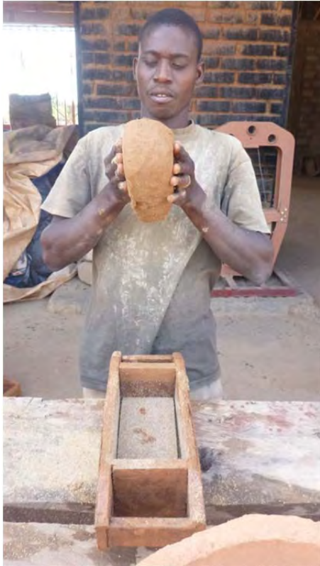
FIGURE 46 - HAND MOULDING BRICKS AT THE PHW FACTORY
