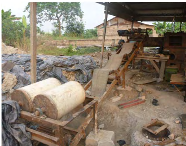
FIGURE 8 - CRUSHER AND CONVEYOR SYSTEM USED TO MOVE CLAY-RICH SOIL TO PUG MILL
