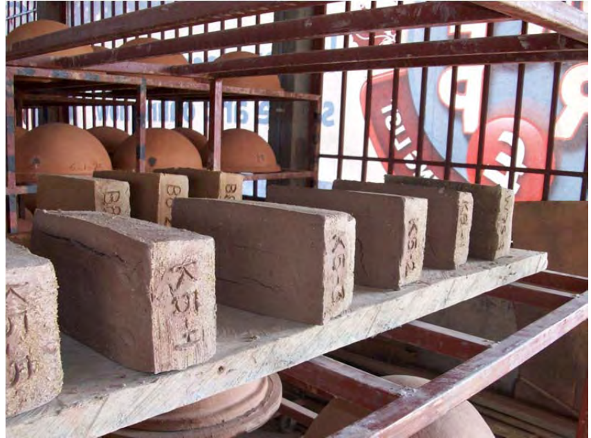
FIGURE 47 - DRYING GREEN BRICKS AT THE PHW FACTORY
